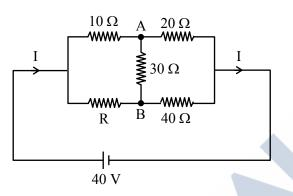
$V_{\text{A}}$  =  $V_{\text{B}}$   $\Longrightarrow$  the bridge is balanced
